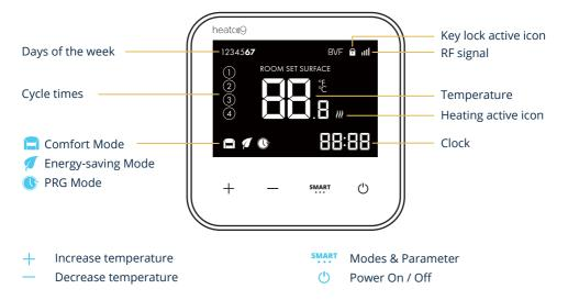
With mains power supply provided, the BVF Heato9 thermostat can be turned on by momentarily touching the right side lower button () once. Depending on the settings, the following values will appear on the display:
