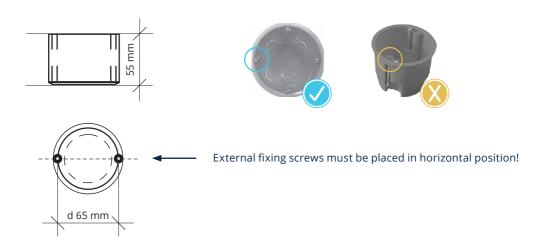
The mounting box should always be of the screw type and be prepared for use with horizontally positioned mounting bolts. The thermostat should be installed in the following manner:
