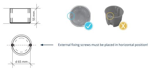
The mounting box should always be of the screw type and be prepared for use with horizontally positioned mounting bolts. The thermostat should be installed in the following manner:
