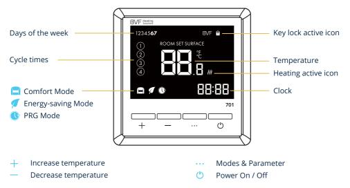
With mains power supply provided, the BVF 701 thermostat can be turned on by pressing the right side lower button () once. Depending on the settings, the following values will appear on the display:
