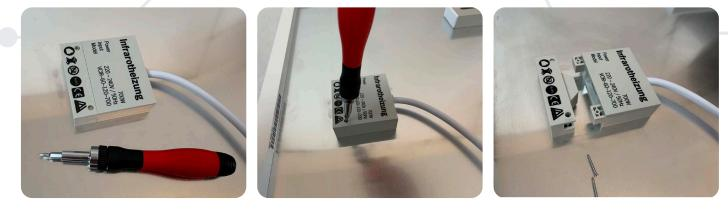
3. Connect the 24-P receiver according to the picture below. Fix it with the screwdriver included in the packaging.
