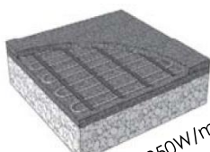
B) Embedded in ASPHALT
