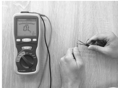
**Heating film resistance test**
